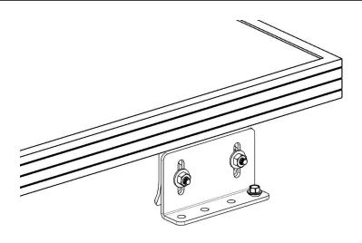
Orient panel in level/plumb layout as desired before fixing in position.
